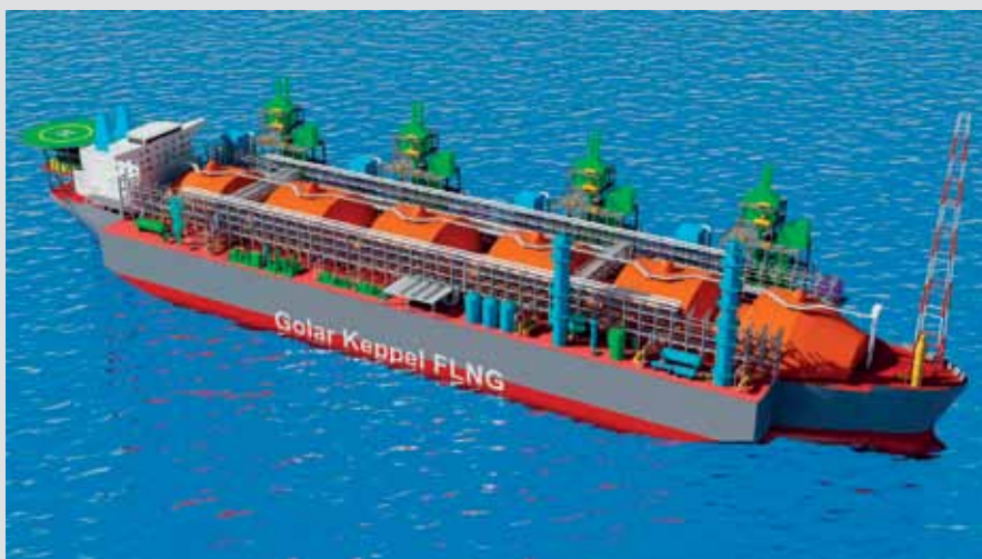
Golar LNG, Keppel Shipyard and Black & Veatch are working together to perform the world's first-of-its type conversion of an existing Liquefied Natural Gas carrier into a Floating Liquefaction Vessel which will offer a faster and more cost effective liquefaction solution when it is completed in early 2017
